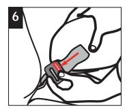
**To remove LATCH:** Remove child from child restraint. Press down firmly on adjuster side of child restraint and press release button to release tension. Unhook LATCH from bar by squeezing spring lever and twist hook.
